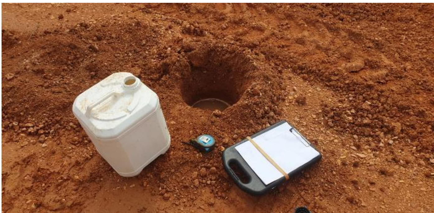
Photograph 12: Infiltration testing in progress near TP25
