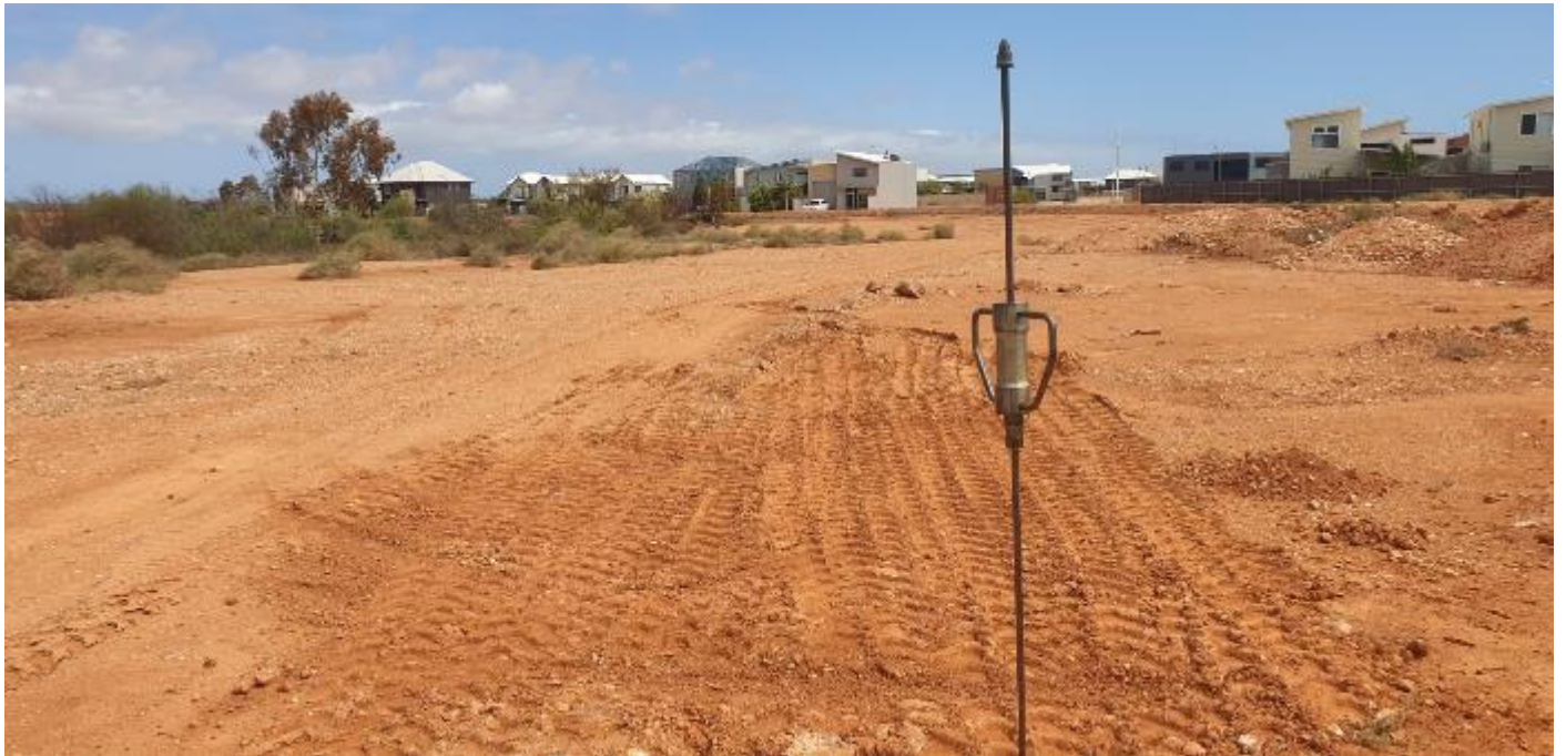
Photograph 13: Facing north from near TP20. DCP testing in progress
