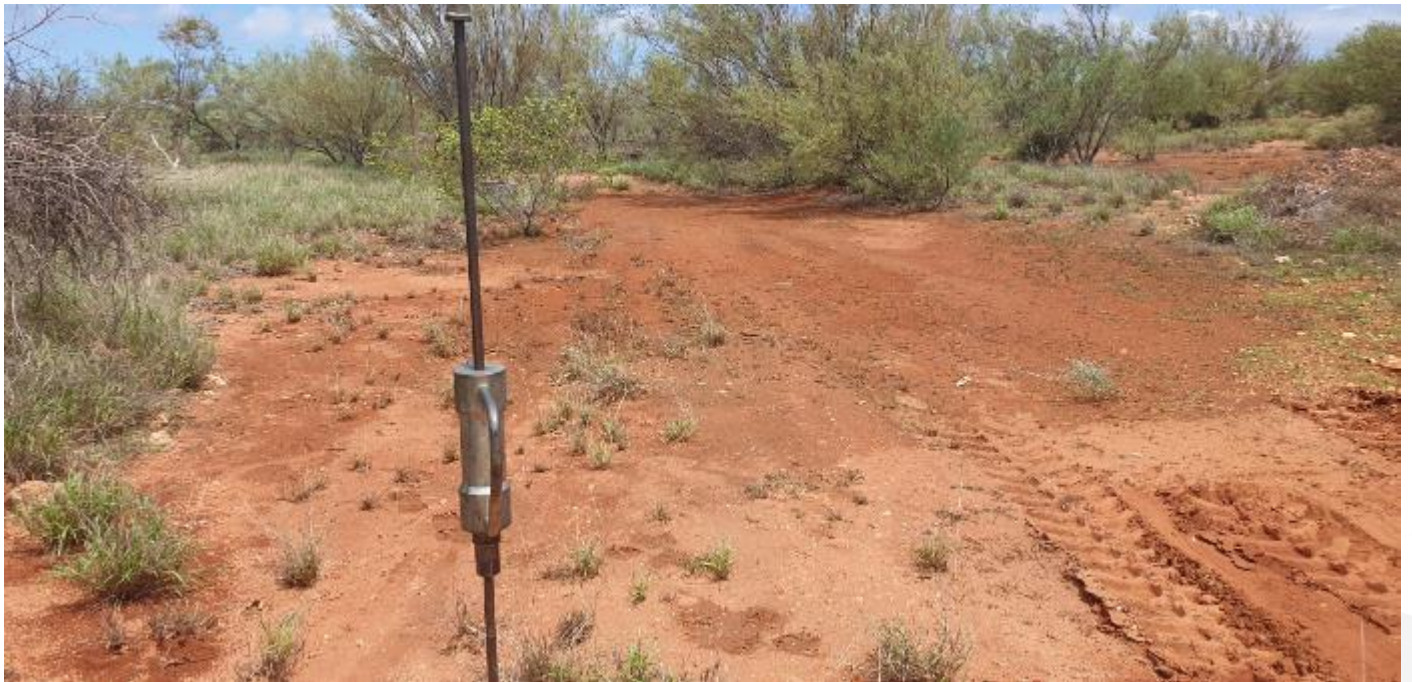
Photograph 14: Facing west from near TP12. DCP testing in progress.
